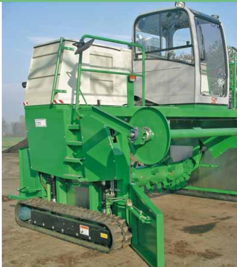
The self-propelled compost turner SG 3400/4000 distinguishes itself by the optimal blending action, which supports the natural structure of the compost materials. Thus proper aeration of the compost windrow is guaranteed, which results in an optimal composting process.
